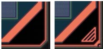
Picture 3: Corner stress relief suggested ( seal ring )
